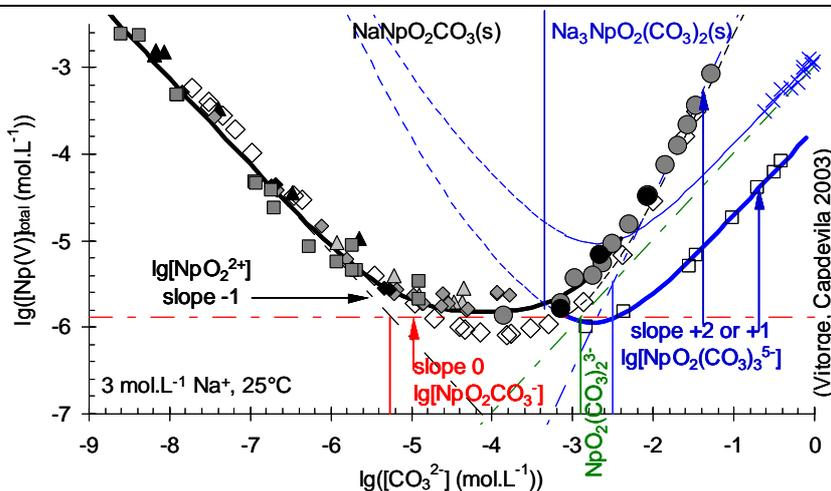
**Figure 2: Np(V) solubility in  $\text{CO}_3^{2-} / \text{HCO}_3^- / \text{CO}_2$  aqueous solutions.**
