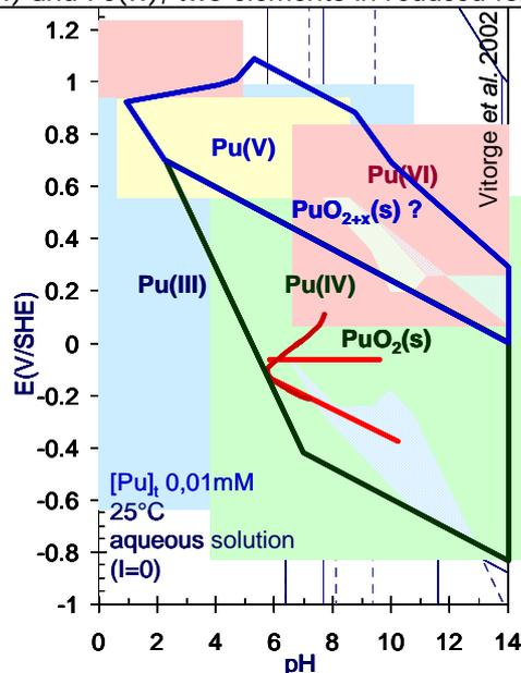
**Figure 10: Pourbaix diagramme for Pu**
